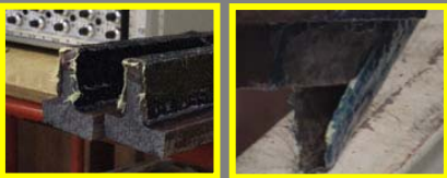
Four point bending test Beams failure modes
